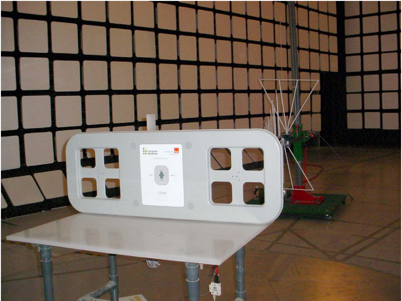
Radiated Emissions at 3m Distance
