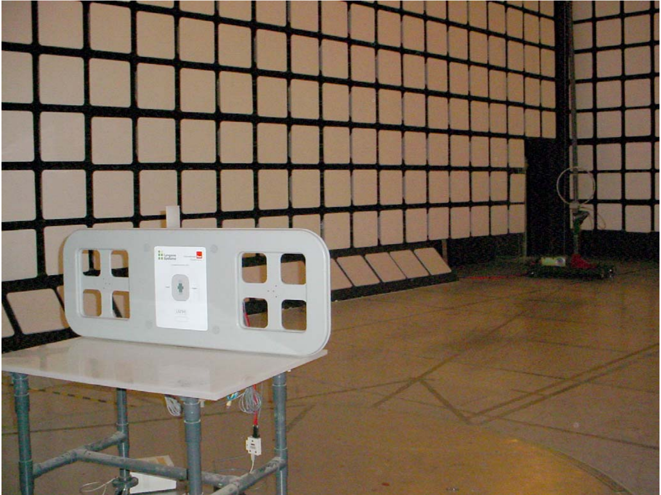
Radiated Emissions at 10m Distance
