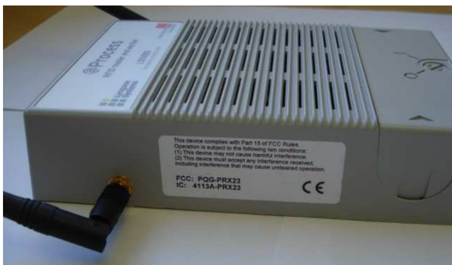
Figure 2 – PRX23 FCC/IC/EC label location
