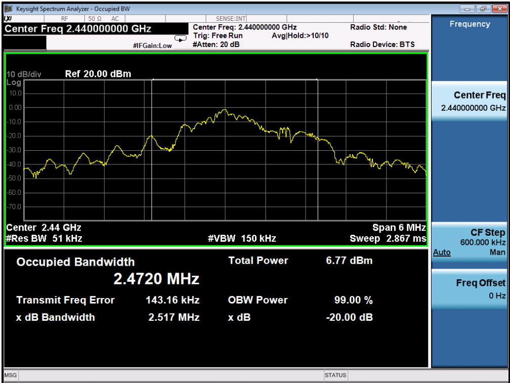
TEST PLOT OF BANDWIDTH FOR MIDDLE CHANNEL
