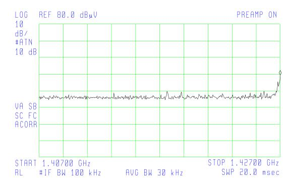
Plot shows lower band edge on right and 20 MHz window. A peak measurement of  $49.40~\rm dBuV/m$  with a limit of  $54~\rm dBuV/m$  avg, data shows a margin of  $4.60~\rm dB$ .
