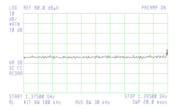
Plot shows lower band edge on right and 20 MHz window. A peak measurement of 41.31~dBuV/m with a limit of 54~dBuV/m avg, data shows a margin of 12.69~dB.
