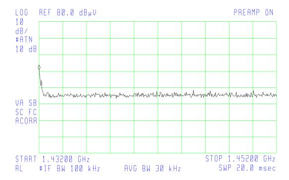
Plot shows upper band edge on left and 20 MHz window. A peak measurement of 50.61 dBuV/m with a limit of 54 dBuV/m avg, data shows a margin of 3.39 dB.
