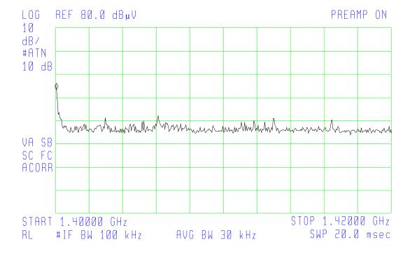
Plot shows upper band edge on left and 20 MHz window. A peak measurement of 53.34~dBuV/m peak, 33.34~dBuV/m Avg with a limit of 54~dBuV/m avg, data shows a margin of 20.66 dB.
