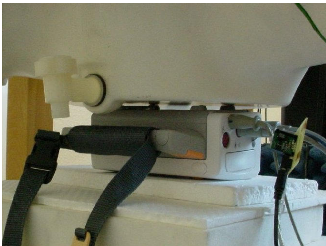
Photo 10: Test position body worn rear side without any distance
