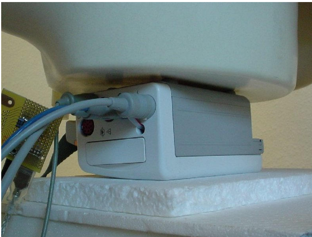
Photo 12: Test position body worn left side without any distance
