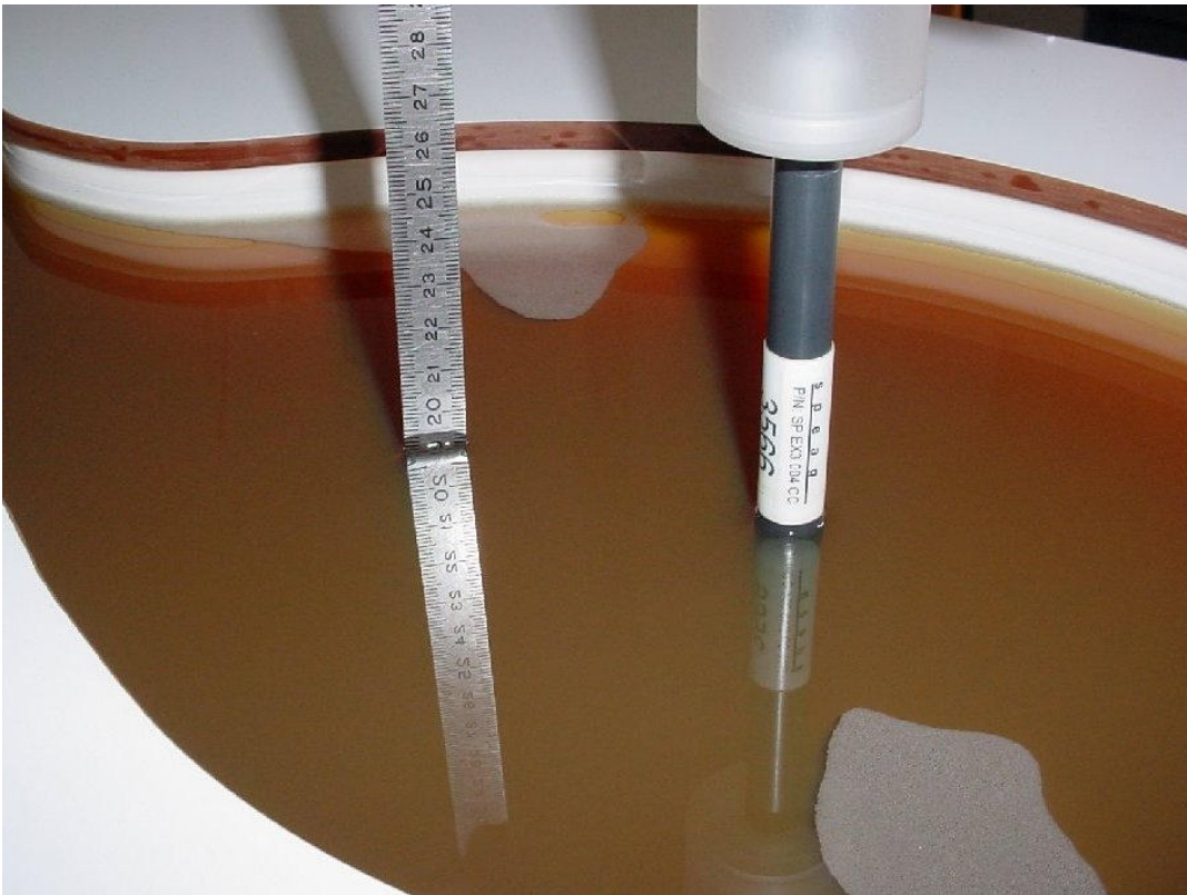
Photo 14: Liquid depth 5 GHz body simulating liquid
