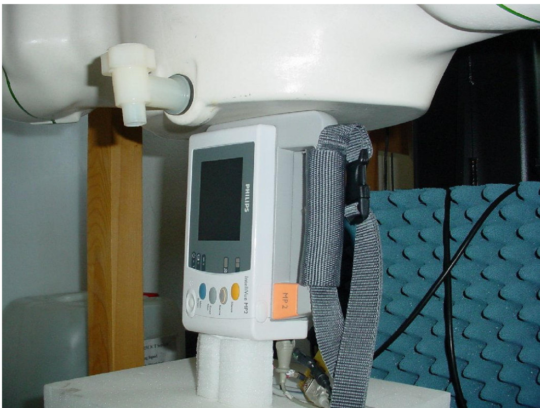
Photo 12: Test position body worn left side without any distance
