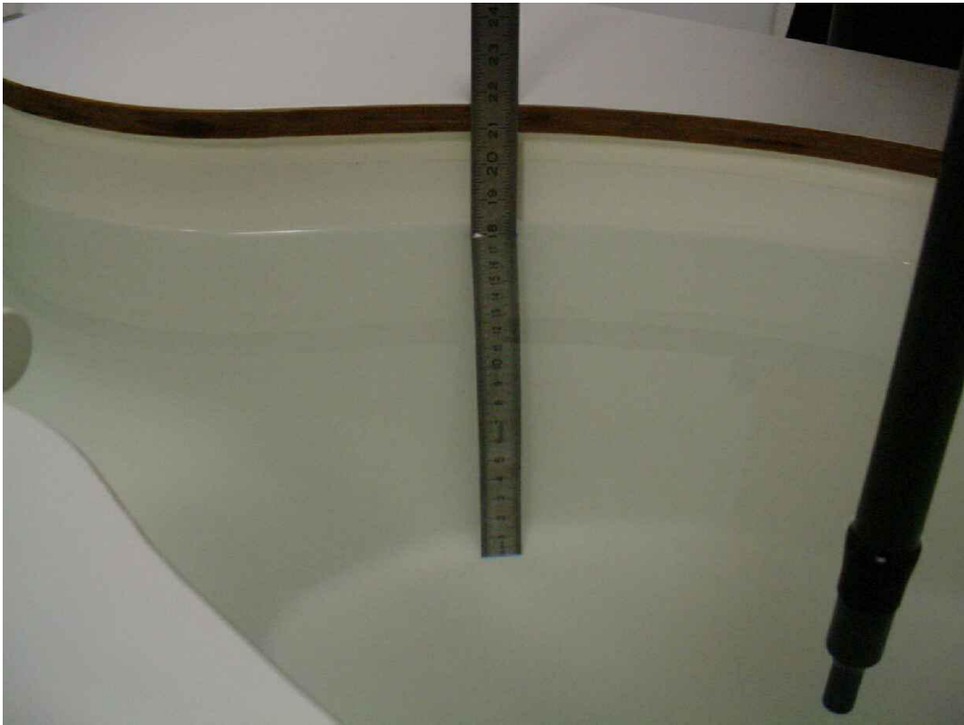
Photo 14: Liquid depth 5 GHz body simulating liquid
