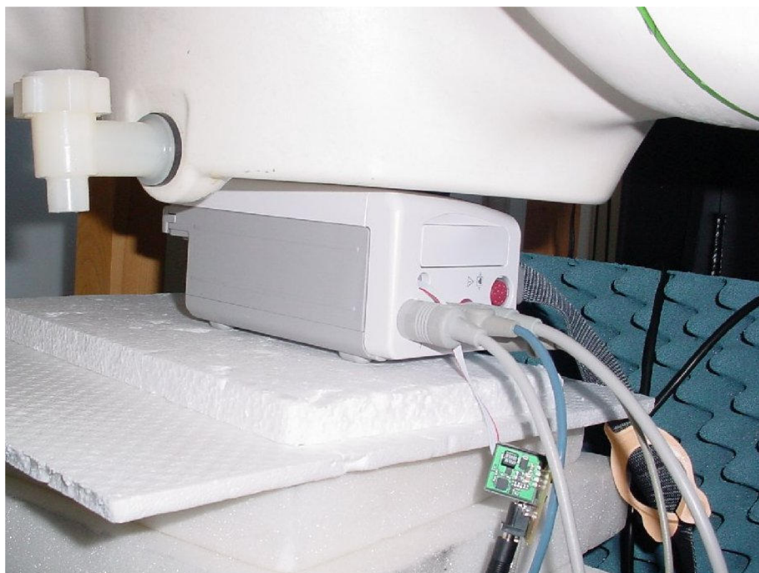
Photo 8: Test position body worn front side without any distance
