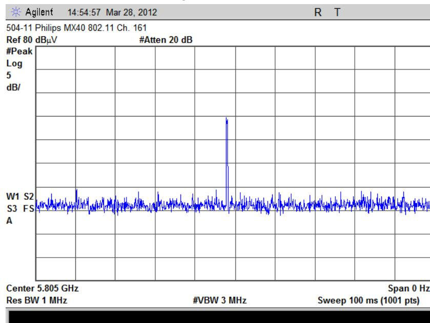
7.11.2 Determination of time averaged output power – Pulse width = 400  $\mu$ s.
