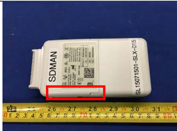
Test Position-2 (LCD-Down with 0mm distance)
