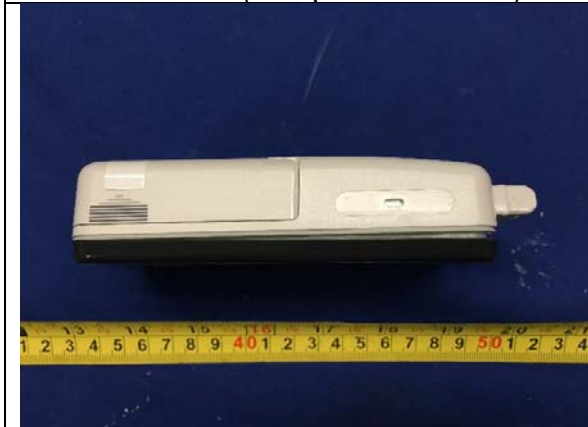
Test Position-3 (Left Side with 5mm distance)
