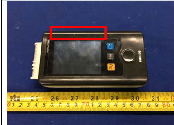
Test Position-1 (LCD-Up with 5mm distance)
