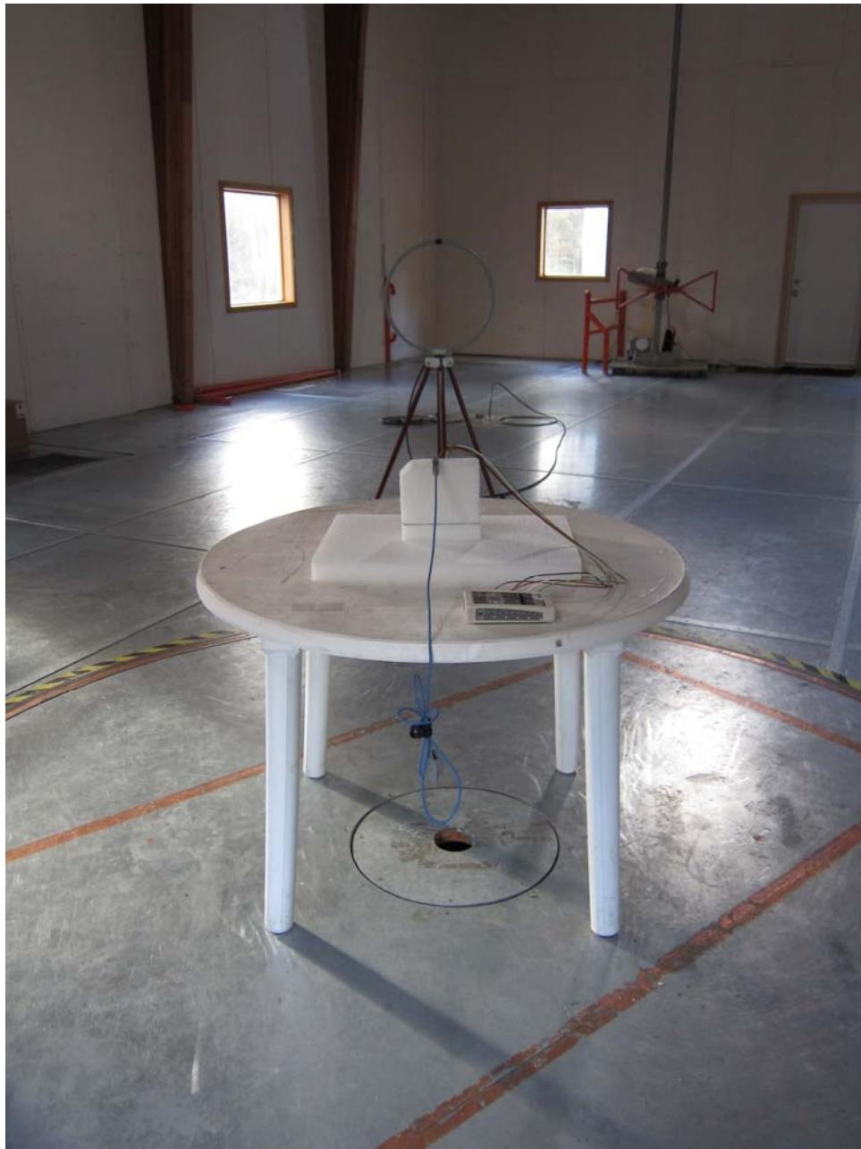
**8. Test Setup Images****8.3. Radiated Emissions – Rear View 30 MHz to 1 GHz**
