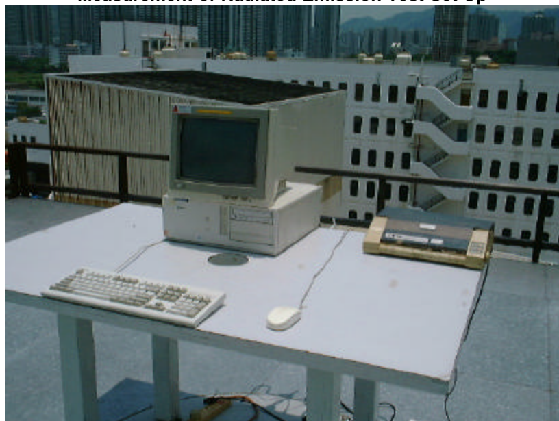
Measurement of Radiated Emission Test Set Up
