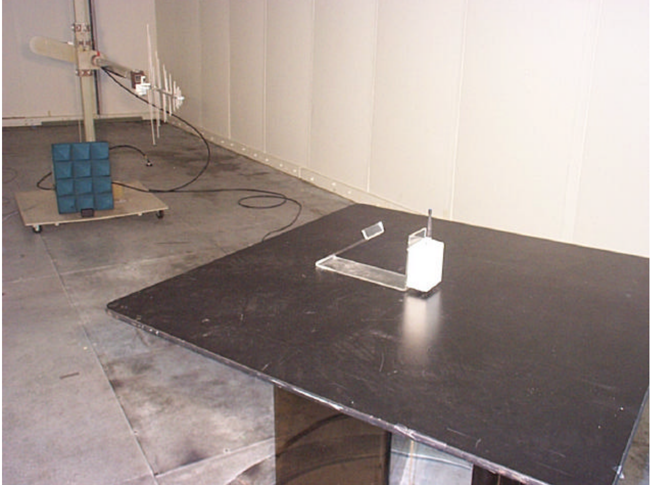
Remtrol, Inc. Wireless Data Relay MCW4 Tested for Spurious Emissions at the OATS Frequency range: 200 MHz – 1.0 GHz
