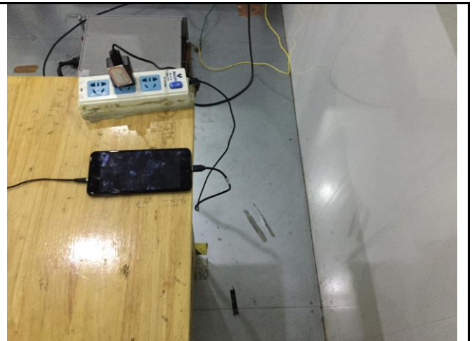
Conducted Emissions Test Setup Side View
