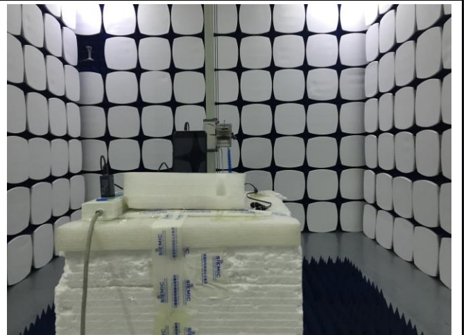
Radiated Spurious Emissions Test Setup Above 1GHz
