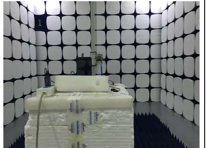
Radiated Spurious Emissions Test Setup Above 1GHz
