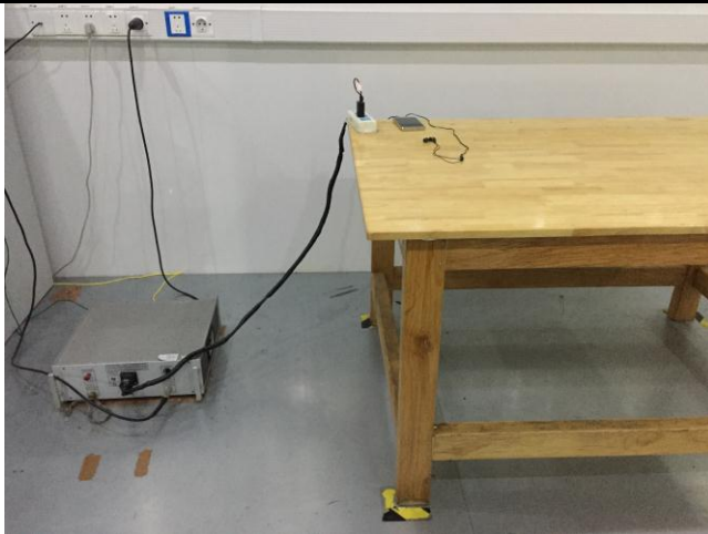
Conducted Emissions Test Setup Front View
