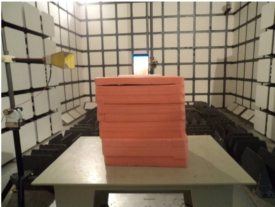
Radiated Emissions Test View (Above 1 GHz)
