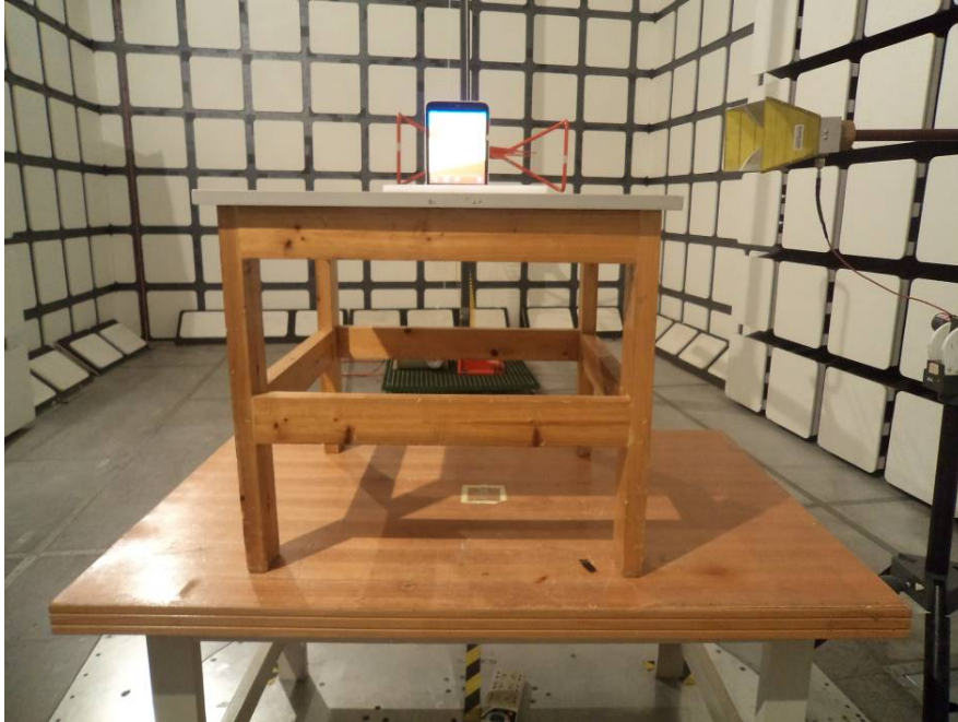
Radiated Emissions Test View (Below 1 GHz)
