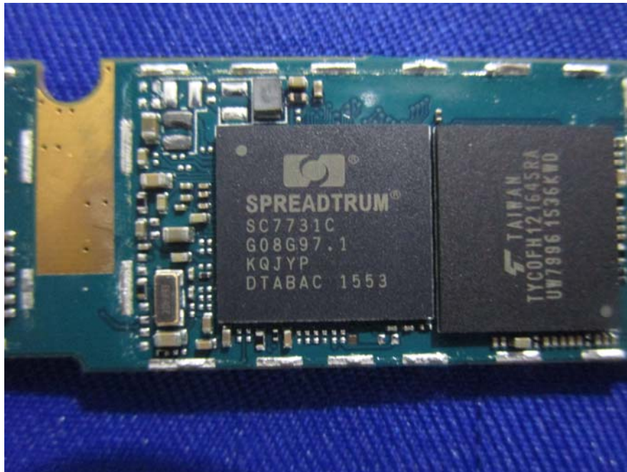
EUT –Main Chip View
