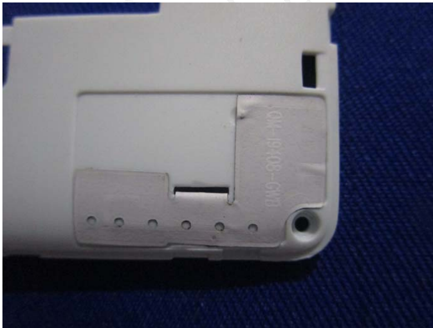
EUT –BT & Wifi & GPS Antenna View
