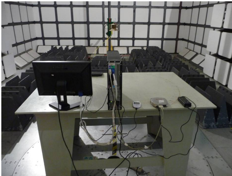
Radiated Emissions – Rear View (Above 1 GHz)
