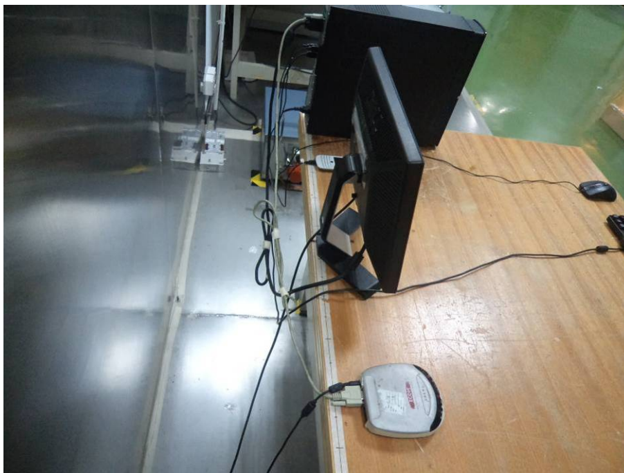
Conducted Emissions - Side View (Downloading mode)
