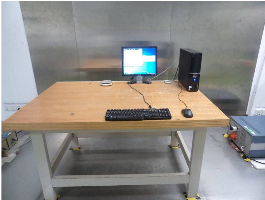
Conducted Emissions - Front View (Downloading mode)
