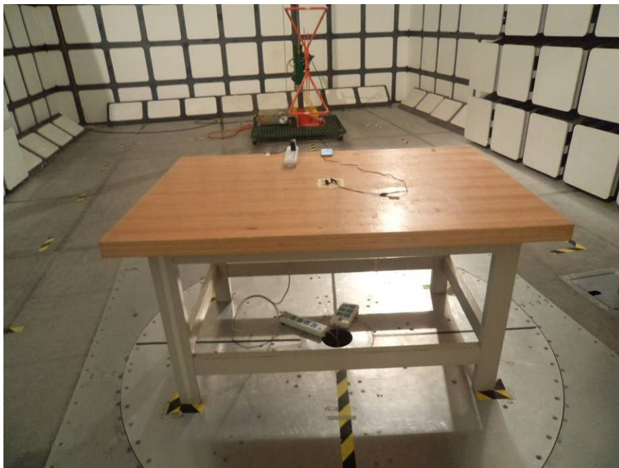
Radiated Emissions-Front View (Charging&multimedia playing mode)
