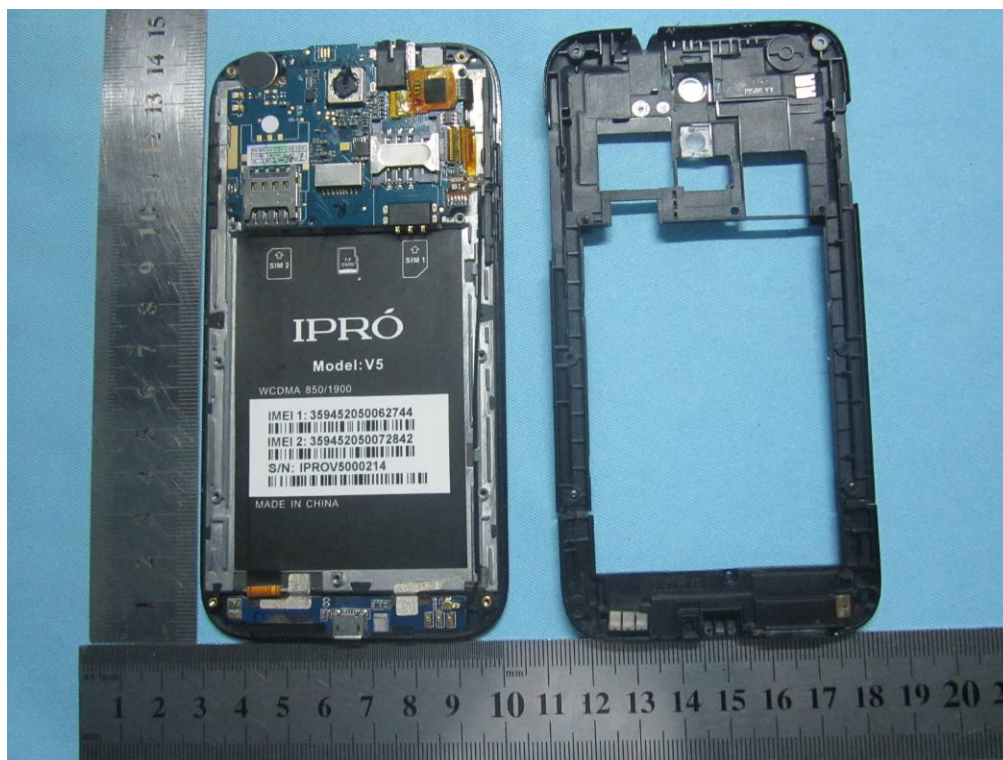
Cover Off - Rear Housing View
