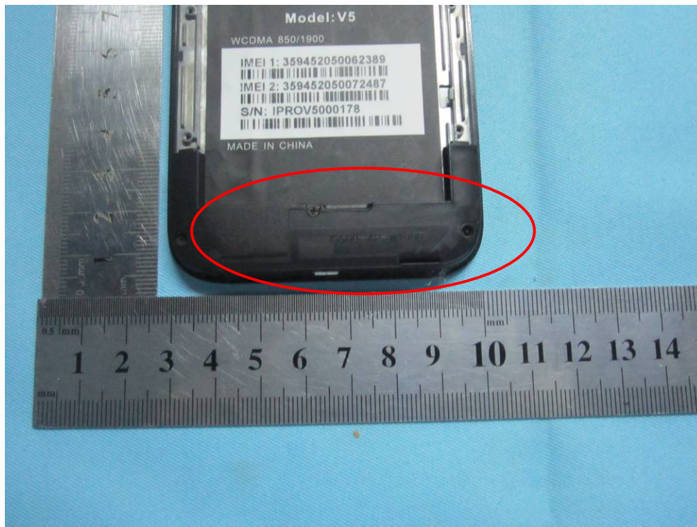
GSM / PCS/ UMTS Antenna View
