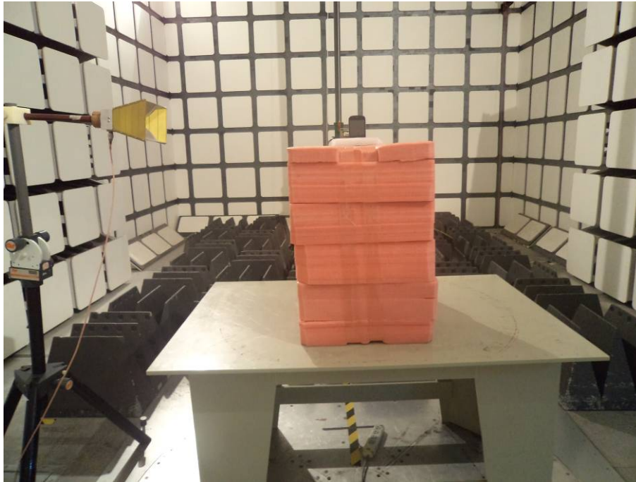
Radiated Emissions Test View (Below 1 GHz)
