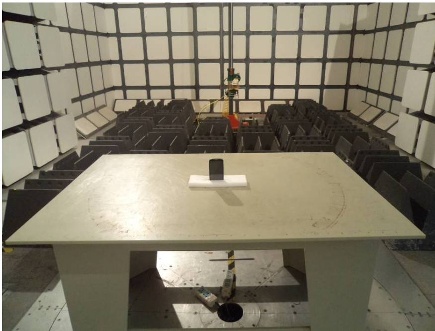
Radiated Emissions View (Above 1 GHz)
