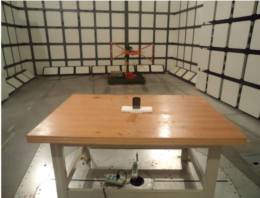
Radiated Emissions View (Below 1 GHz)
