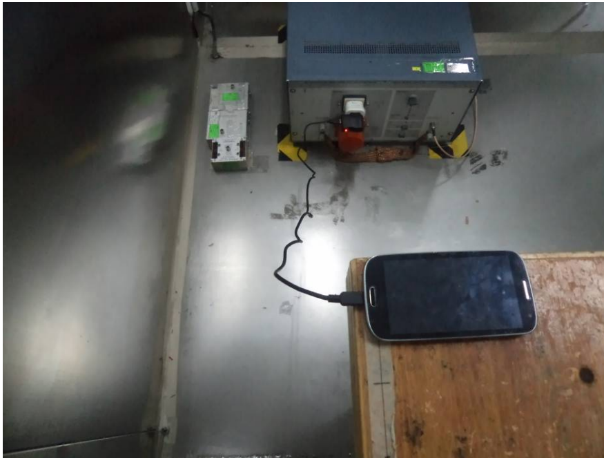
Conducted Emissions - Side View
