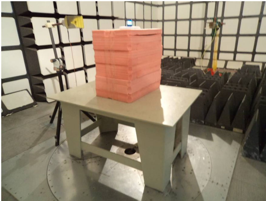
Radiated Emissions Test View (Above 1 GHz)
