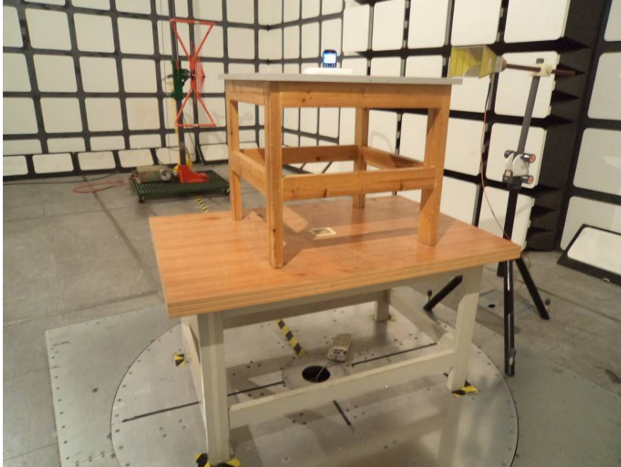
Radiated Emissions Test View (Below 1 GHz)
