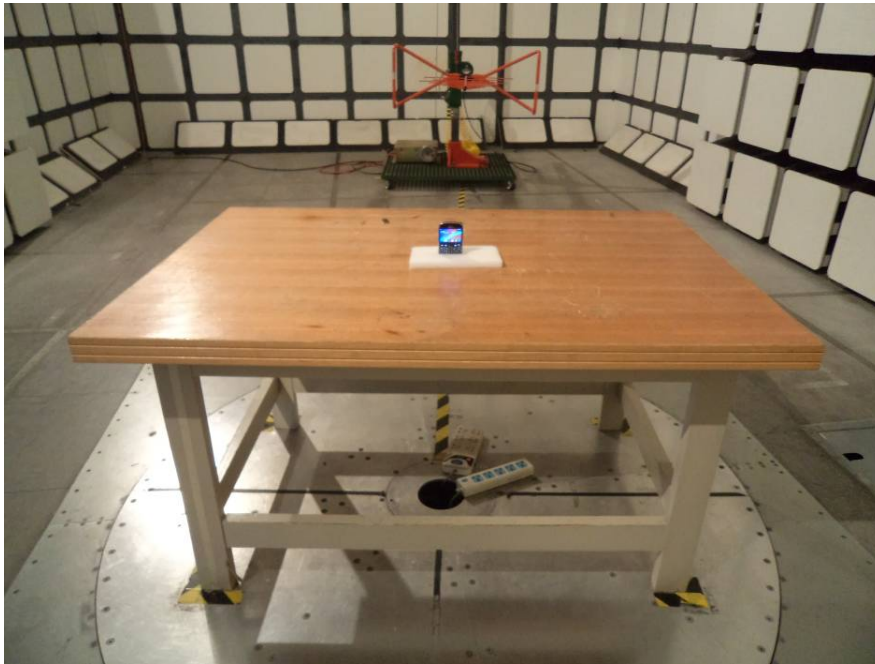
Radiated Emissions View (30-1000 MHz)
