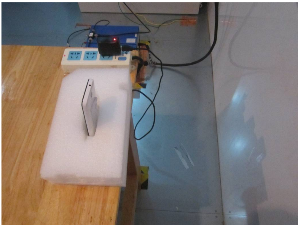
Conducted Emissions Test Setup Side View
