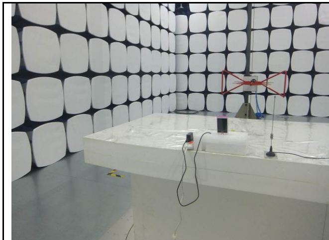
Radiated Spurious Emissions Test Setup Below 1GHz
