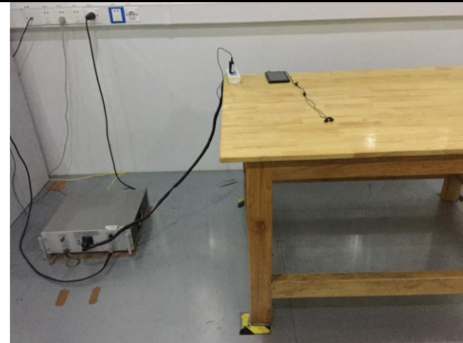
Conducted Emissions Test Setup Front View
