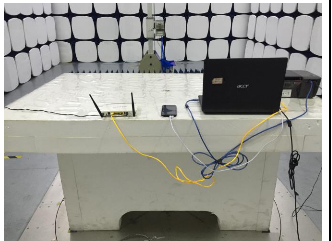
Radiated Emissions Test Setup Above 1GHz
