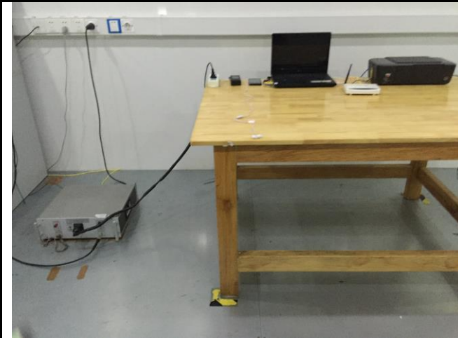
Conducted Emissions Test Setup – Front View
