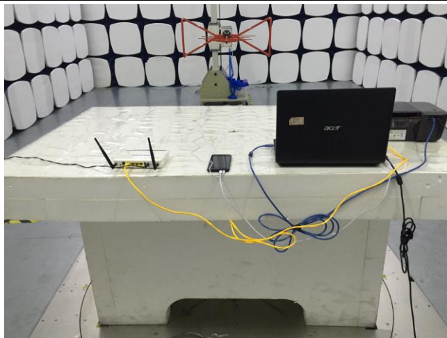
Radiated Emissions Test Setup Below 1GHz
