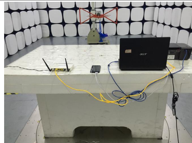
Radiated Emissions Test Setup Below 1GHz
