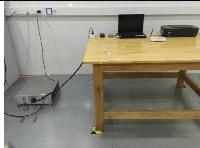
Conducted Emissions Test Setup – Front View
