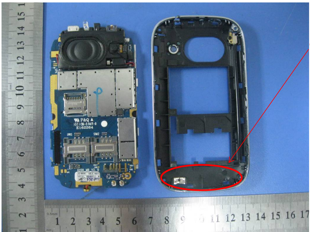
GSM Antenna - Top View
