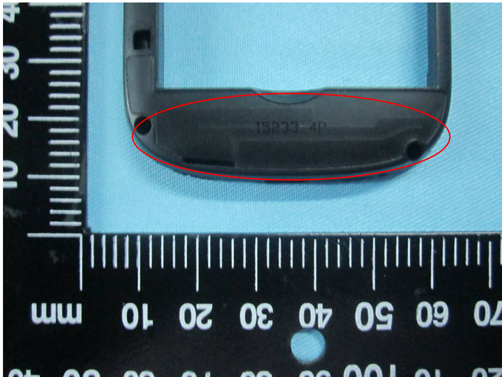
GSM/PCS Antenna View
