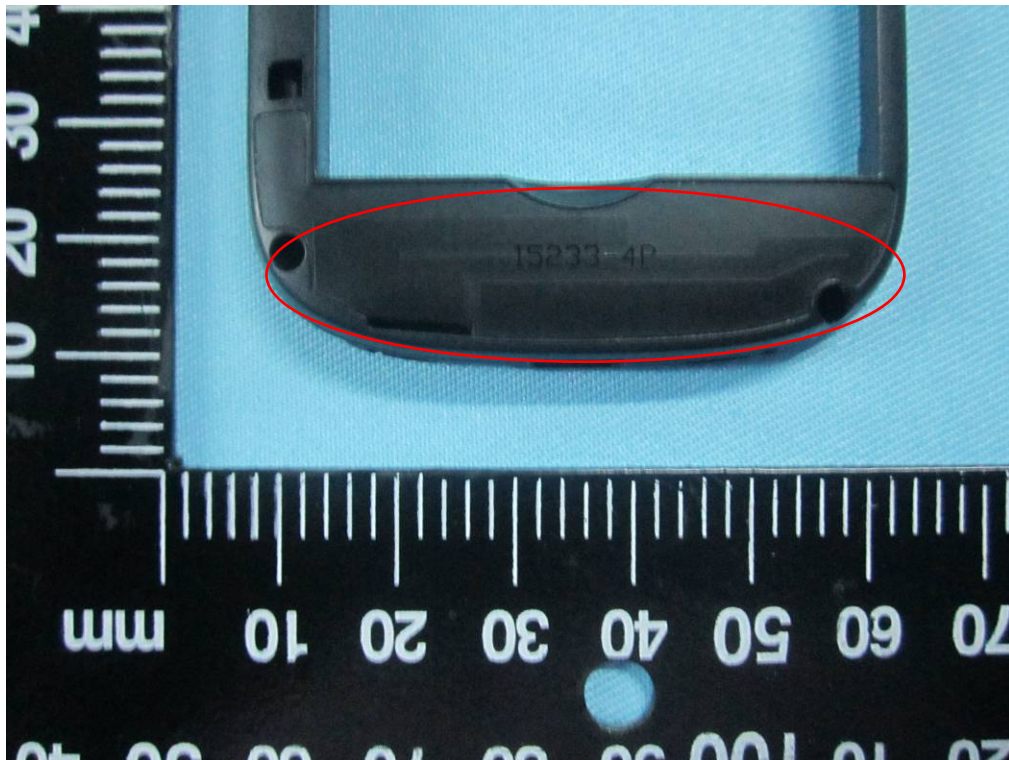
GSM/PCS Antenna View
