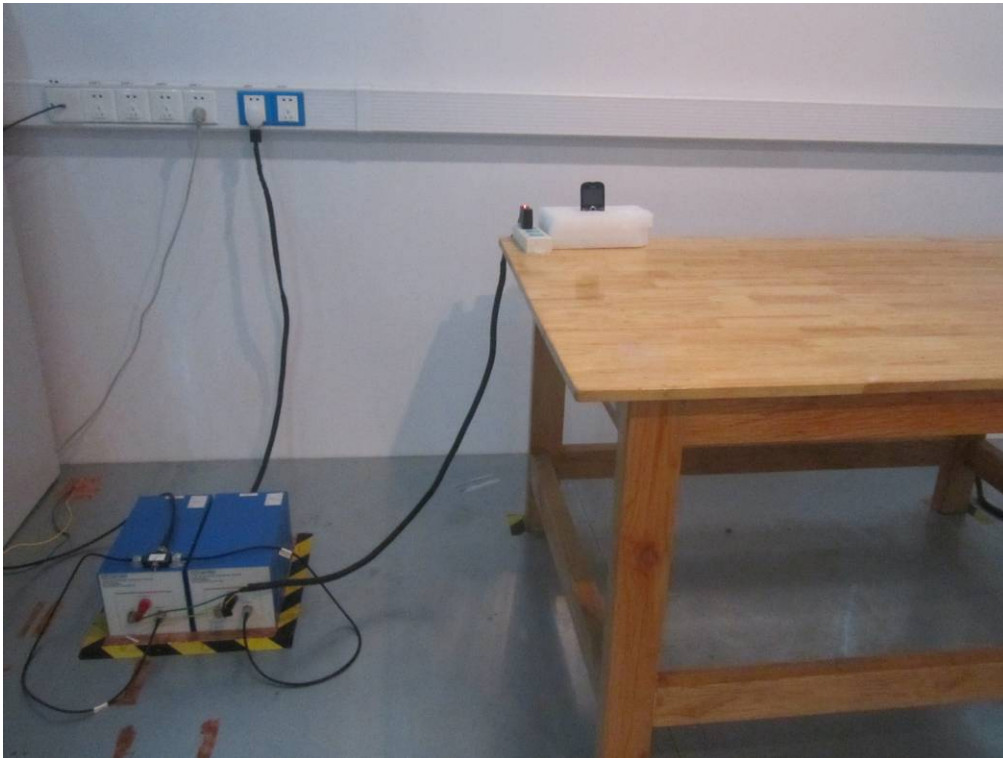
Conducted Emissions Test Setup Front View
