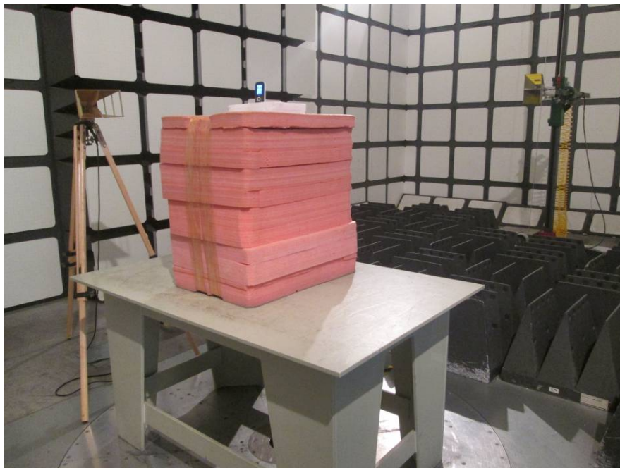
Radiated Emissions Test View (Above 1 GHz)
