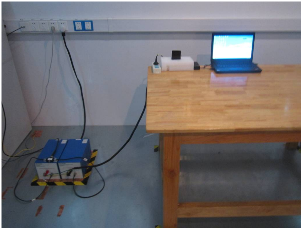
Conducted Emissions Test Setup Front View
