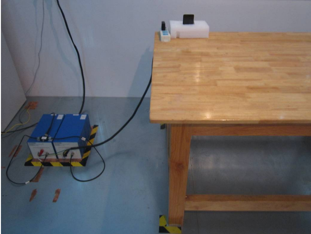
Conducted Emissions Test Setup Front View
