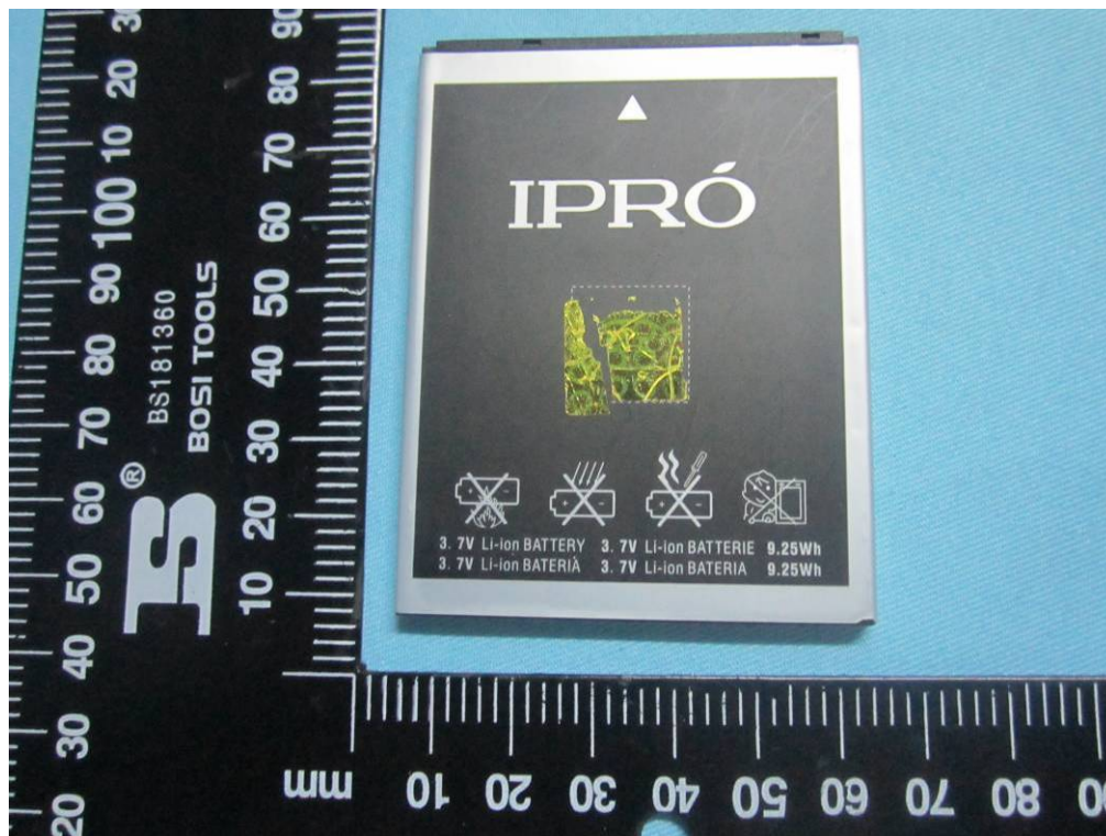
Battery - Top View
