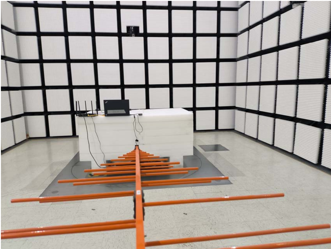
Radiated Emission Below 1GHz Rear View
