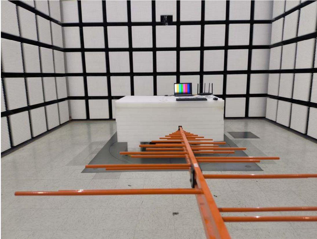
Radiated Emission Below 1GHz Rear View
