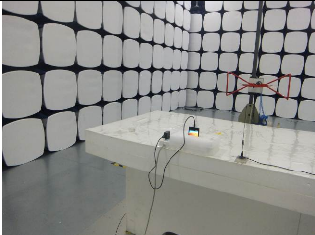
Radiated Spurious Emissions Test Setup Below 1GHz
