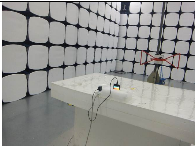
Conducted Emissions Test Setup Front View
