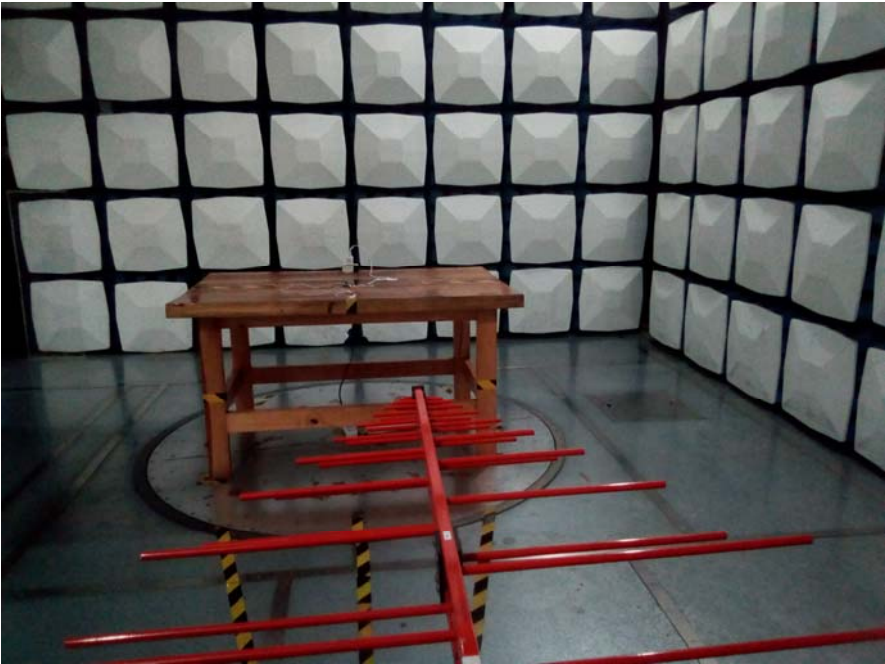
Radiated Emission Below 1GHz View
