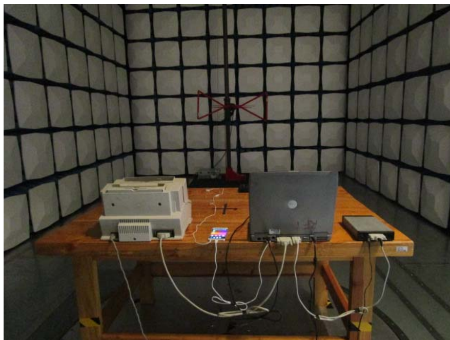
Radiated Emissions –Rear View (Below 1GHz)
