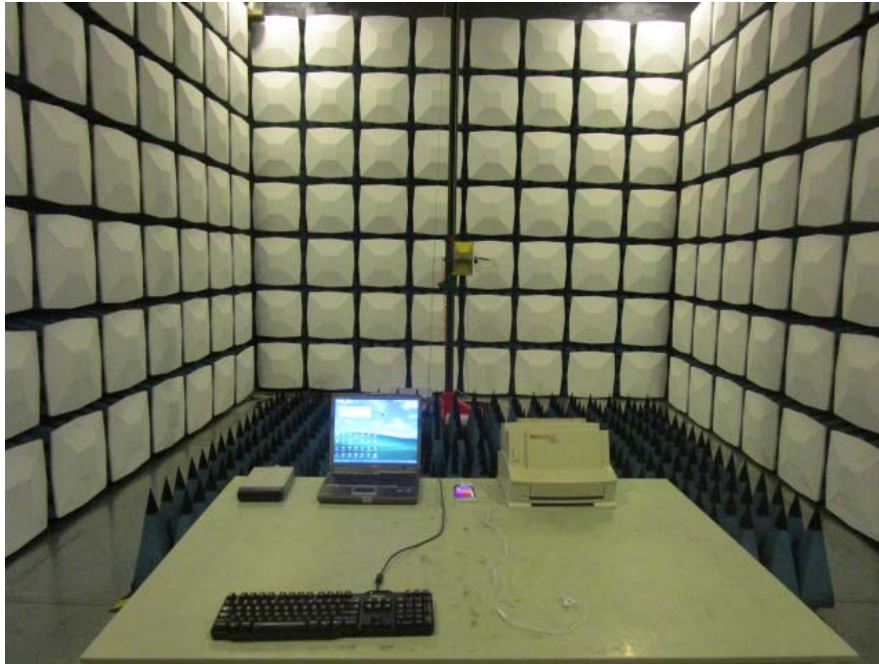
Radiated Emission –Front View (Above 1 GHz)
