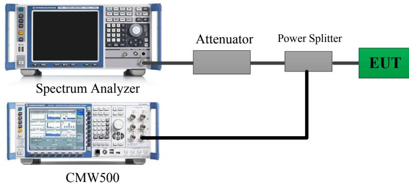
A short RF cable with low cable loss connected to the EUT antenna port, which was provided by manufacturer. The cable loss of this RF cable was offset into the setting of test equipment, which was provided by manufacturer ▲.
