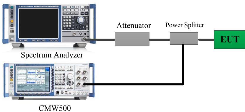
A short RF cable with low cable loss connected to the EUT antenna port, which was provided by manufacturer.
