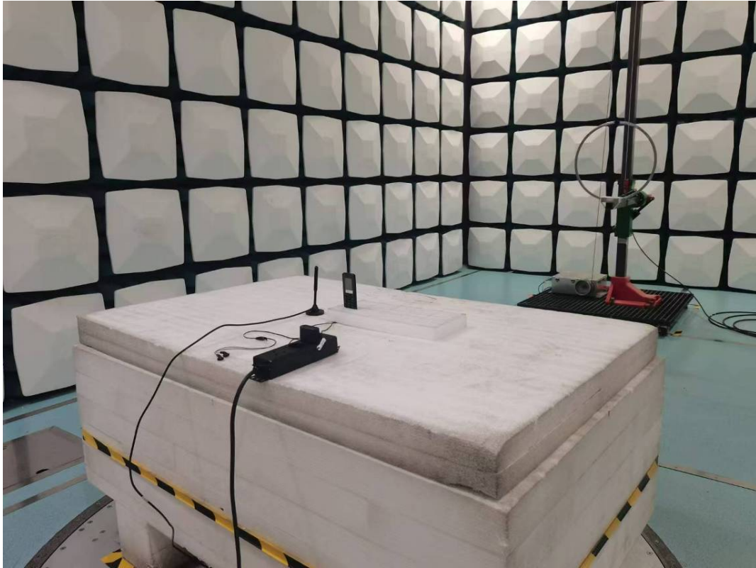
Radiated Emission 9k-30MHz Perpendicular View
