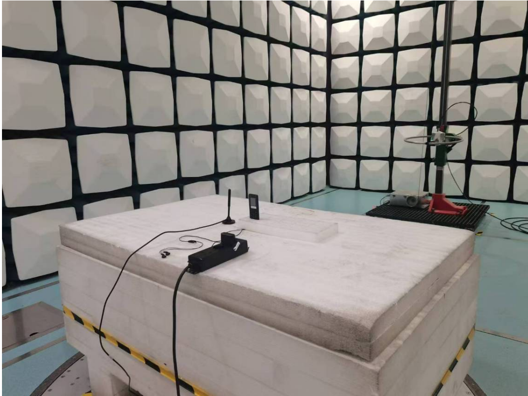
Radiated Emission 30M-1GHz View
