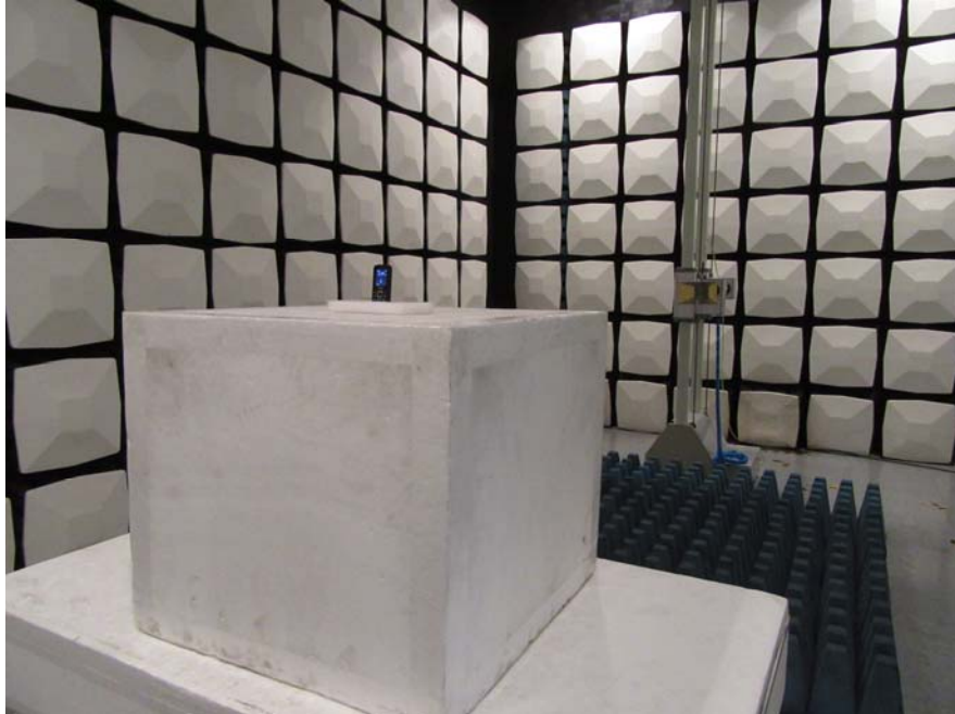
Radiated Emission View (Above 1GHz)
