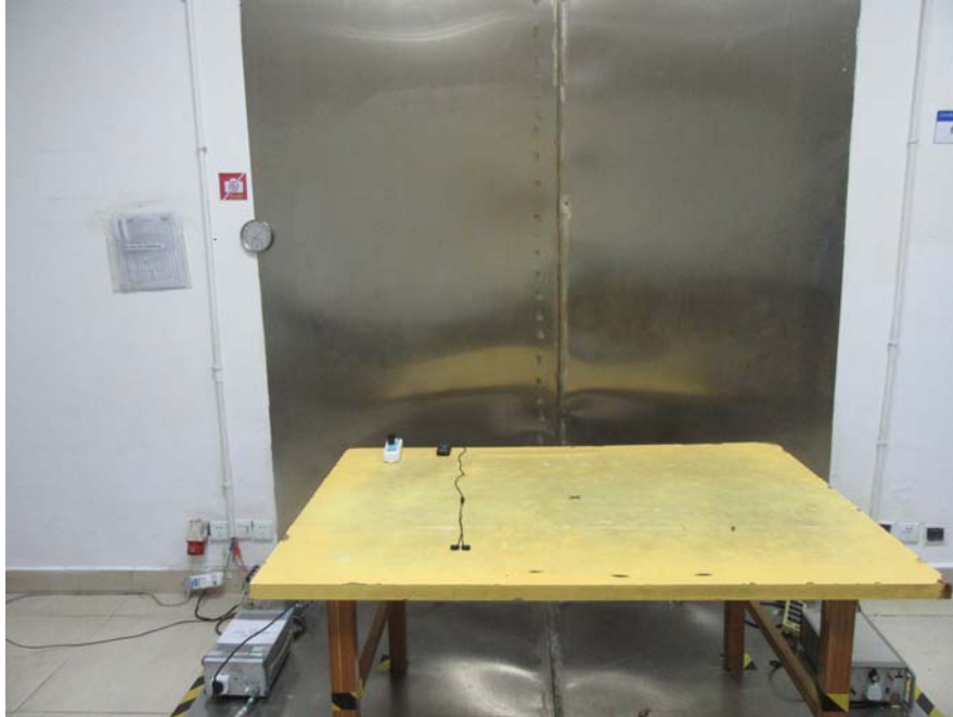
Conducted Emissions – Front View
