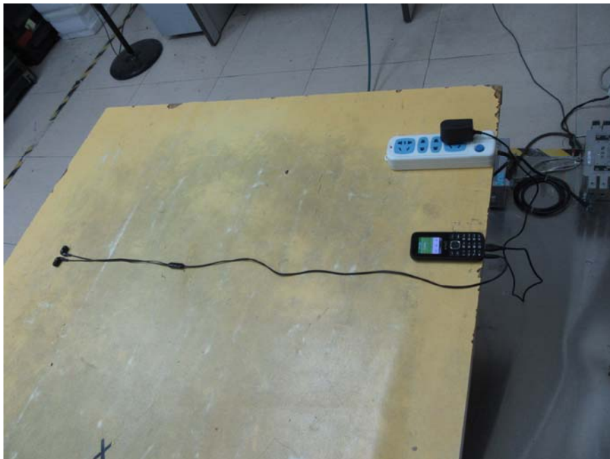
Conducted Emissions – Side View
