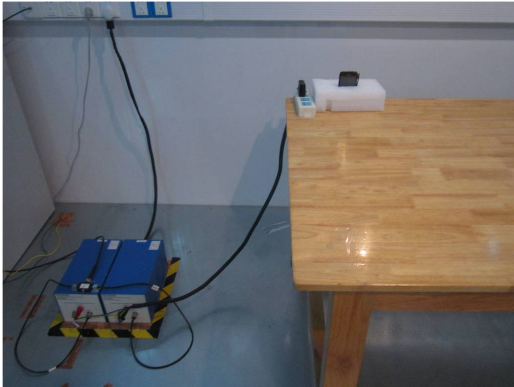
Conducted Emissions Test Setup Front View
