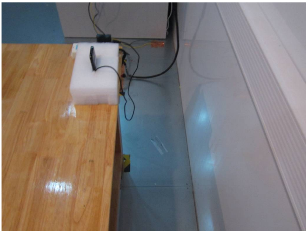
Conducted Emissions Test Setup Side View
