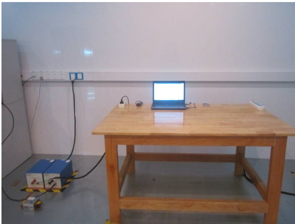
Conducted Emissions Test Setup Front View
