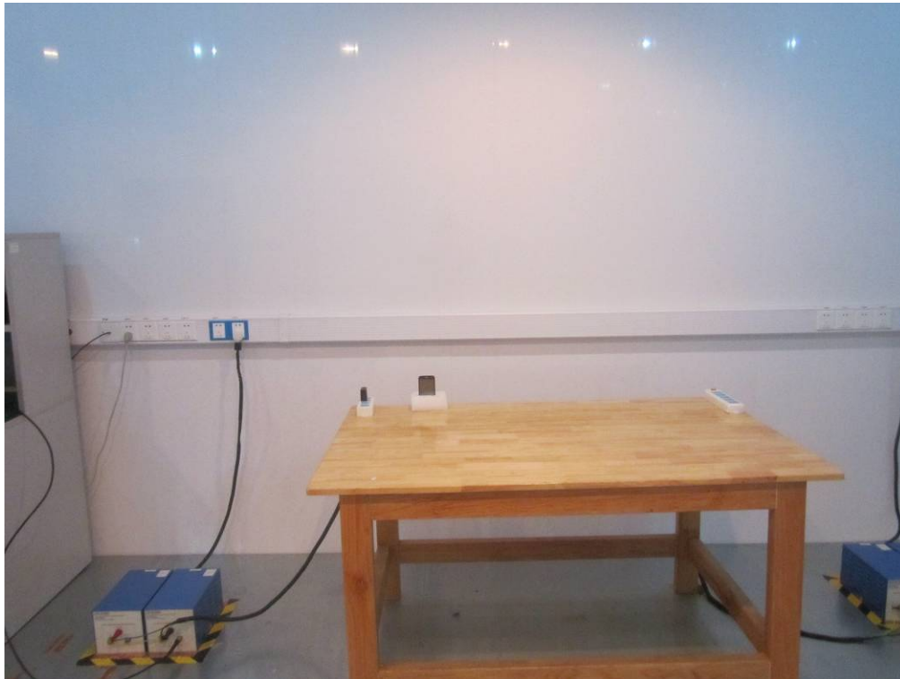
Conducted Emissions Test Setup Front View
