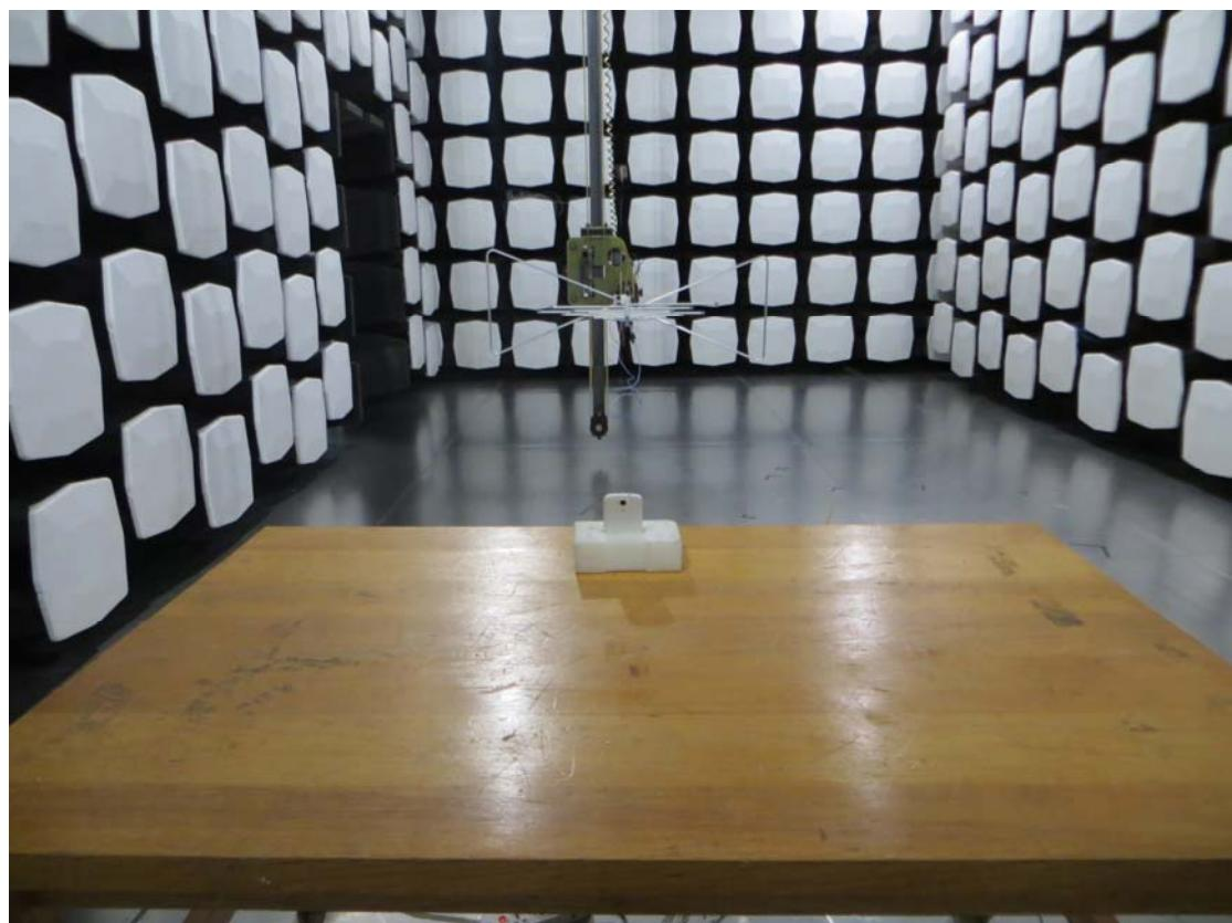
2. Part 15C Radiated emission above 1GHz
