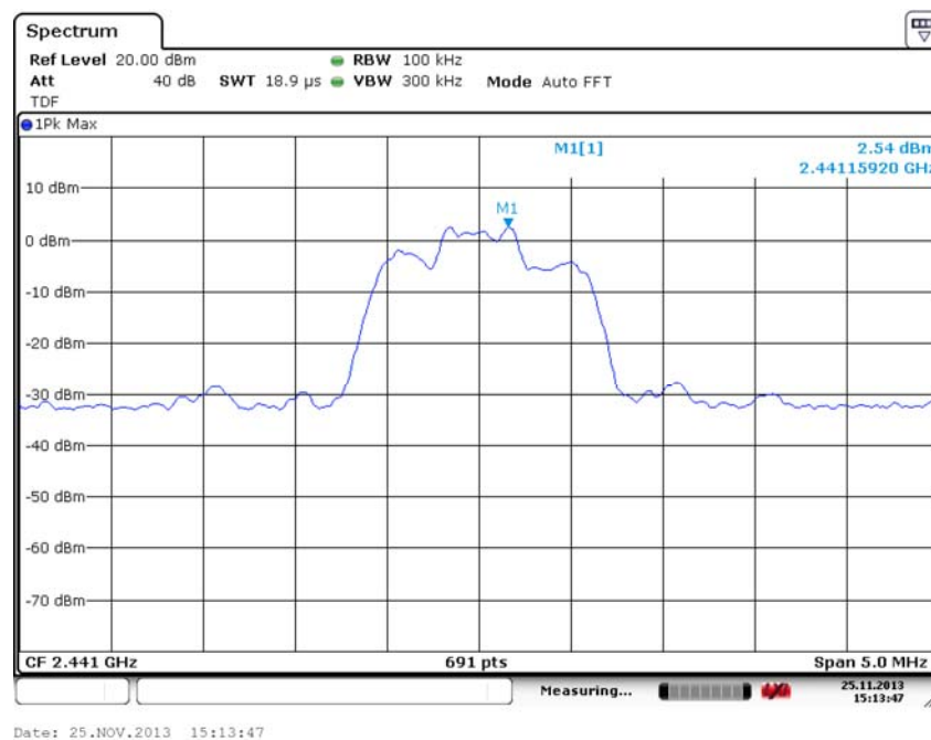
Fig. 34 Conducted Spurious Emission (8DPSK, Ch39, 2.441GHz)
