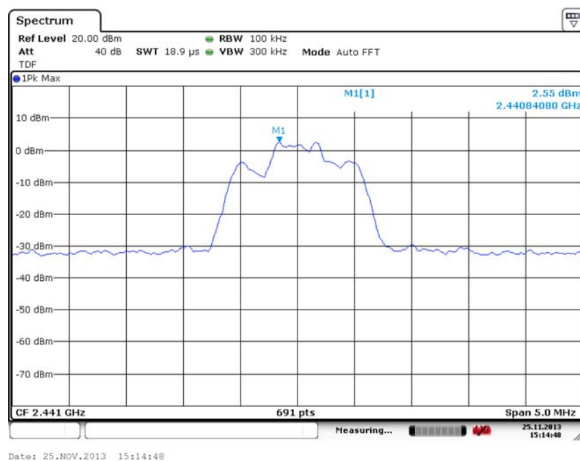
Fig. 25 Conducted Spurious Emission ( \pi/4 DQPSK, Ch39, 2.441GHz)
