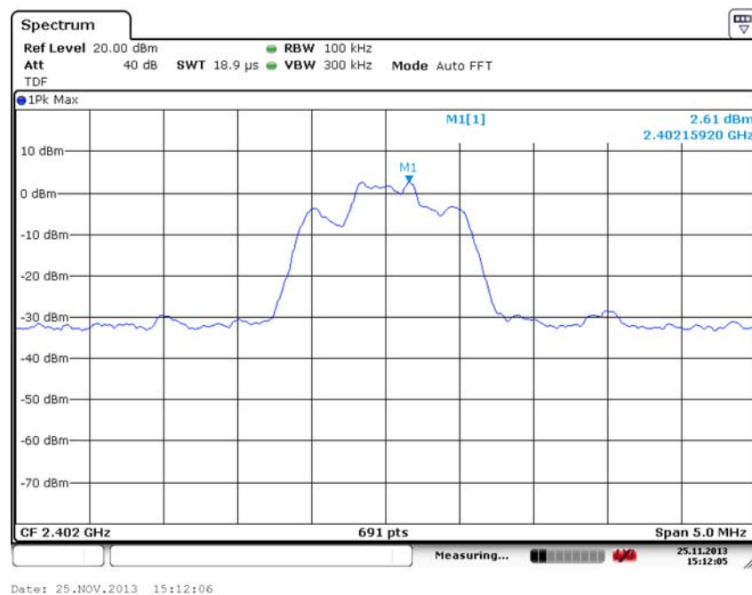
Fig. 22 Conducted Spurious Emission ( \pi/4 DQPSK, Ch0, 2.402GHz)
