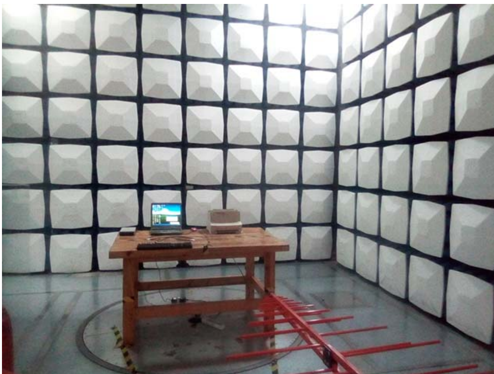
Radiated Emissions Below 1G front View
